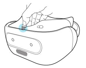
**3.** Insert the microSD card, with the gold contacts facing out, into the slot.
