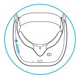
Press the Volume buttons on the bottom left side of the headset or the right side of the controller to adjust the volume.
